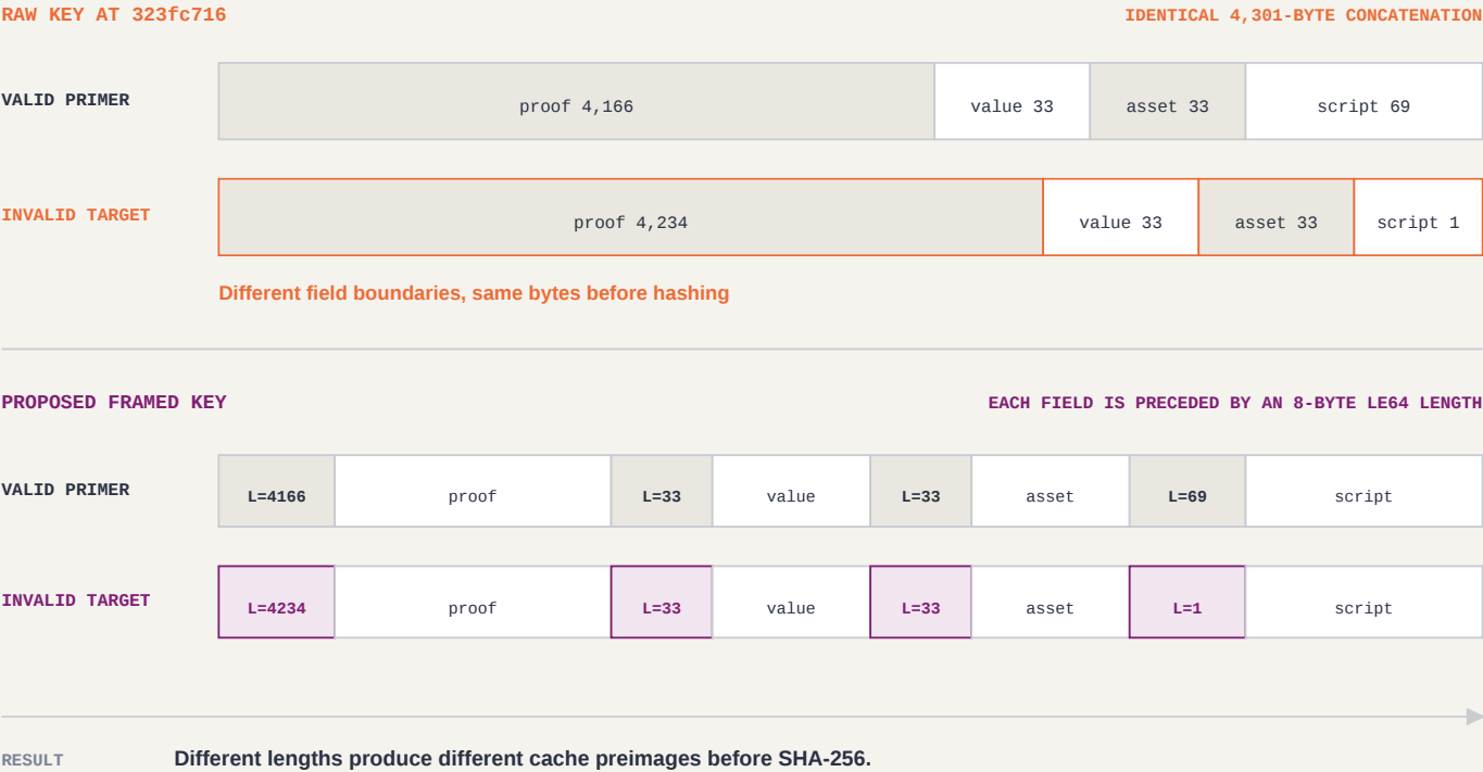
Figure 2. The current key hashes an untyped byte stream. The repair writes an LE64 length before every field, so moving bytes across a boundary changes the preimage before hashing.
